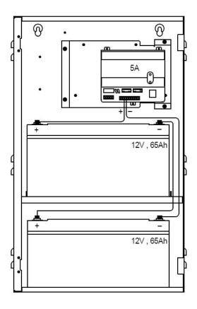
WARNING – Always fit 2 batteries and wire in series, the product will not work correctly with a single 12V battery.
