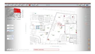
In a fire event, the seat of the fire is uniquely identified and time stamped and subsequent fire alarms are time stamped, allowing the operator to see where the fire has started and where and how quickly it is spreading. In addition the status the air handling units, smoke spill and stair pressurisation fans can be monitored to show the spread of smoke.
