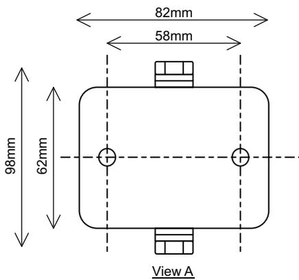
2off - Fixing holes 6.25mm (0.25") Dia.
