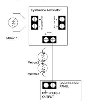
Figure 9: Typical Igniting Actuator Circuit Wiring
