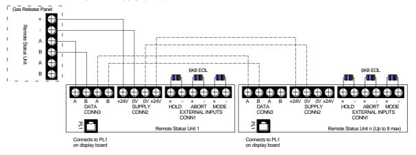
Figure 10: Typical RSU Circuit Wiring
