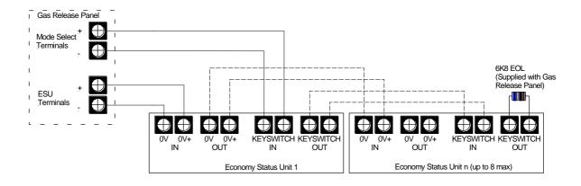
Figure 11: Typical ESU Circuit Wiring
