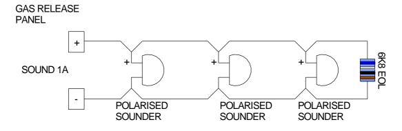
Figure 5: Typical Sounder Circuit Wiring
