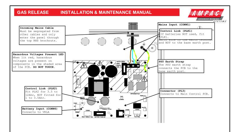
Figure 12: Power Supply PCB Layout and Connection Details
