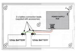
**Note**: The battery connection leads (red lead, black lead and green link wire) are supplied in the accessory pack.
