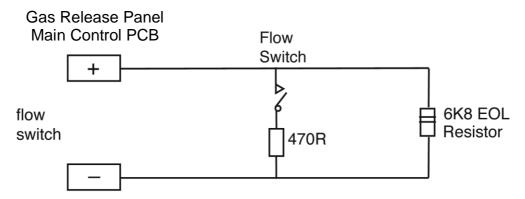
Figure 6: Typical Monitored Input Wiring
