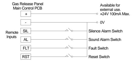
Figure 7: Typical Remote Control Input Wiring
