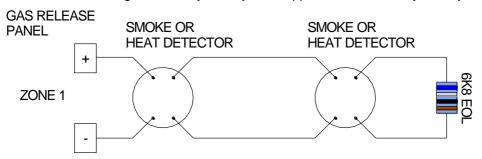
Figure 4: Typical Detector Circuit Wiring
