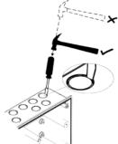
Always ensure that if a knockout is removed, the hole is filled with a good quality 20mm cable gland. Any unused knockouts must be securely blanked off.
