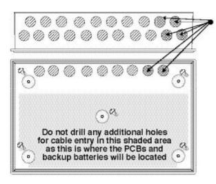
These knockouts are used for incoming mains cable in order to maintain cable segregation.
