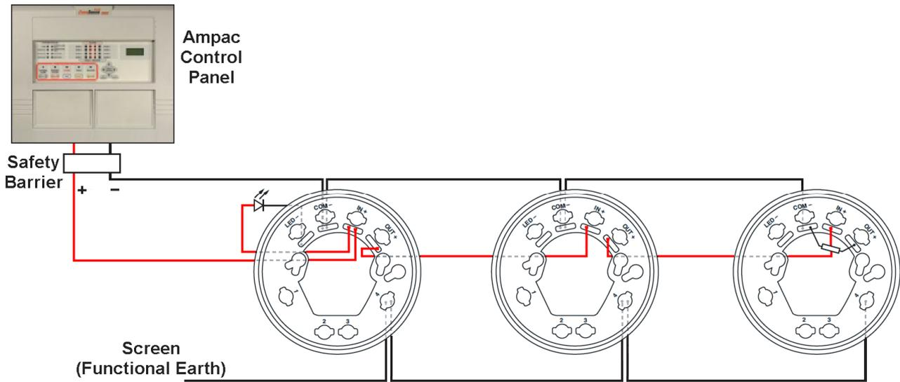
Figure 5 – Orbis IS TimeSaver Base Wiring Diagram
