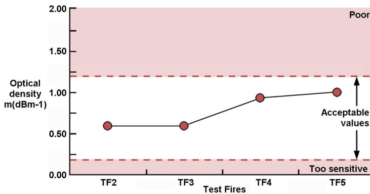
Figure 1 - Orbis Optical Detector Response to Test Fires
