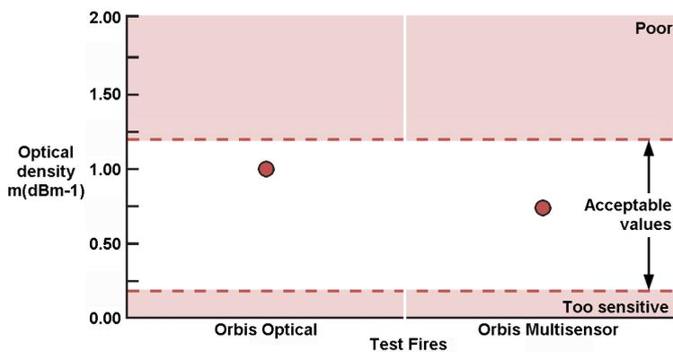
Figure 2 - Comparisons of Response between Orbis Optical & Multisensor
