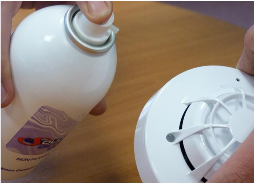
Image A - cleaning a detector with a air pressure canister
