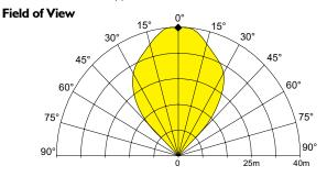
To meet the requirements of EN54:10 clause 5.4, where the ratio of the response points Dmax: Dmin should not exceed 1.41, the horizontal and vertical viewing angles max should not exceed  $\pm 30^{\circ}$ .
