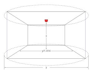
X – The maximum height at which the device may be mounted
