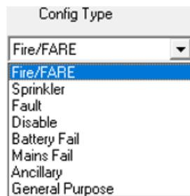
Figure 49: Relays Config Type Selection Options
