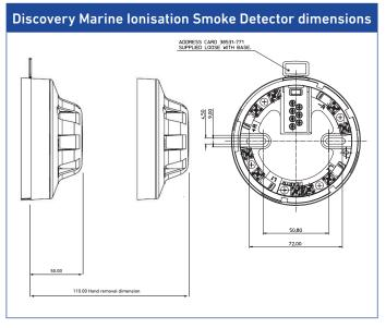
*Note:* Should be used with Deckhead Mounting Box - Part No. 45681-217 if ingress protection is required.
