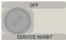
It is a requirement that control be secured from unauthorised use. A keyswitch has therefore been included in the control process.
