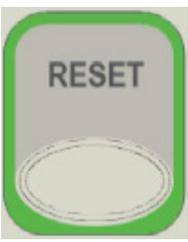
key is pressed to reset the fire condition. All outputs activated in response to the fire will deactivate and the panel will revert to the normal condition providing there are no other abnormal conditions present. The operation of the RESET key will be logged.
