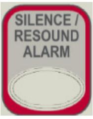
key is pressed to silence any silence-able outputs that have been activated.
