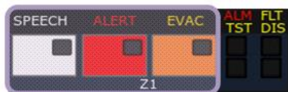
Figure 5-4 Emergency zone with controls highlighted.
