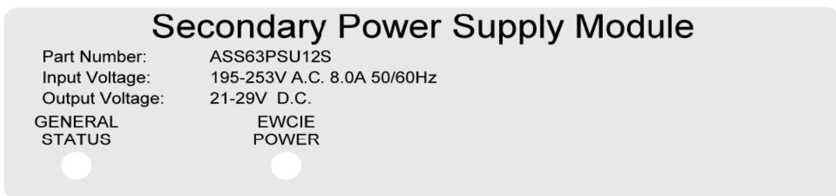
Figure 4-7 Secondary power supply labelling
