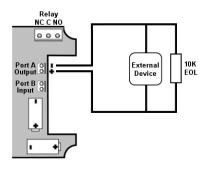
Provides a maximum external drive of 100 mA at 12 Vdc or 50 mA at 24 Vdc. The  $10 K\Omega$  EOL resistor monitors whether the cable has been damaged or the connection is no longer available.
