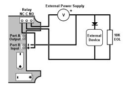
Ensure the device connected to the Output Module is not drawing more than 2A at 30V. Drawing too much current through the output relay or connecting 220/240 ac mains voltage could possibly damage the unit and void warranty.
