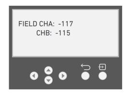
If this screen is showing high levels of RF noise, RF communication with paired devices may be negatively affected and could cause repeated or delayed communication, as well as link faults. This would also negatively affect battery life as a result.
