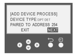
Note: The first product will be auto-assigned as [Hub Address +1], then [Last Assigned Address +1] for each subsequent product paired. These addresses can be changed manually before the system is released.
