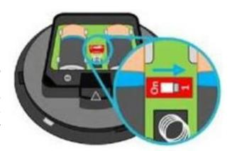
Once the switch is moved, the Loop Interface LCD should display 'DEVICE FOUND'.
