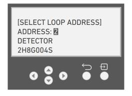
Select the device to be removed by navigating through the assigned device loop addresses using the up and down arrows.
