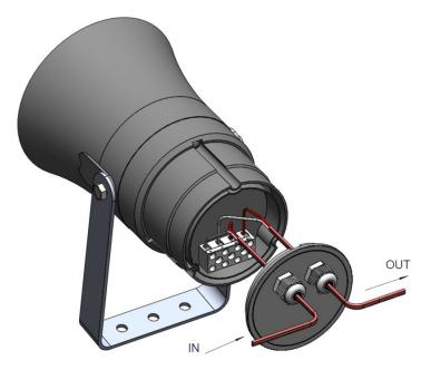
1) Remove the "U' shape bracket from the speaker and position where required on the wall or pole. Mark the fixing points and fix the bracket using suitable fixings (not supplied)
