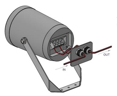
1) Remove the "U' shape bracket from the speaker and position where required on the wall or pole. Mark the fixing points and fix the bracket using suitable fixings (not supplied)
