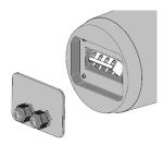
3) Select the desired power tapping using the rotary switch.
