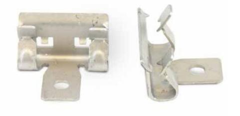
Beam clips may be used to support the LHD cable directly (in this case a separate silicon pad is required) or fixed to other mounting brackets and used to affix the bracket to a RSJ/I-beam or equivalent.
