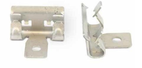
Beam clips may be used to support the LHD cable directly (in this case a separate silicon pad is required) or fixed to other mounting brackets and used to affix the bracket to a RSJ/I-beam or equivalent.
