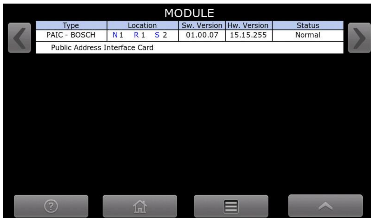
Figure 6-29 PAIC status screen
