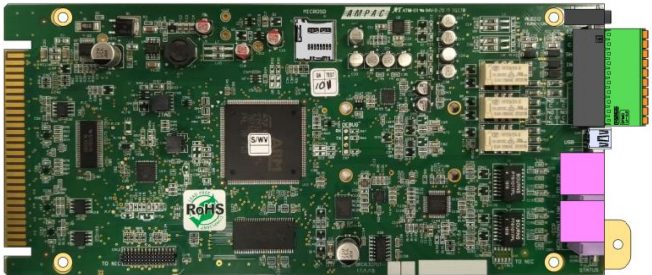
Figure 4-24 Detail of DCPU Card with Audio Jack fitted.
