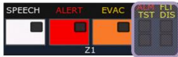
Figure 5-3 Emergency zone with indicators highlighted.
