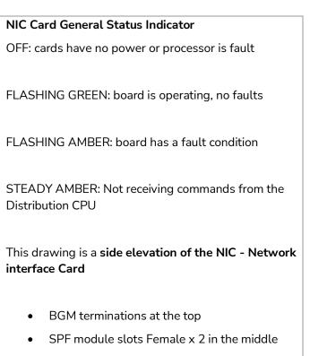
• Ethernet connections at the bottom
