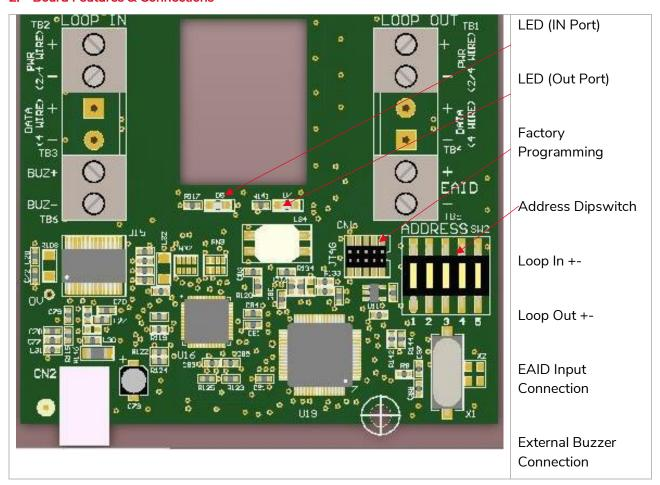
The address dipswitches 1 to 5 from left to right each equal address settings 1-2-4-8-16 respectively Setting address 20 = Both Dipswitch 5 and 3 (16+4) will be placed in the ON (Up Position) Addressing starts from address 1
