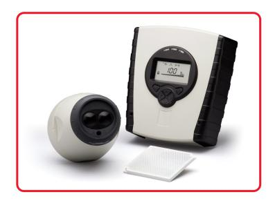
The detector is factory set to a beam obscuration of 35% which is the nest setting for most factories and warehouses. The settings can be changed to 25% for offices and clean areas such as theatres or to 50% for hostile areas such as mills or foundries. The detector reports a Pre alarm (analogue value 480 at the approximately 75% of the alarm threshold.
